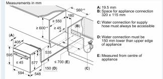
If the appliance will be installed underneath a hob, the following worktop thicknesses (including substructure if necessary)
