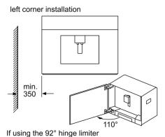
(spare part no. 00636455), the minimum distance to the wall is only 100 mm. measurements in mm
